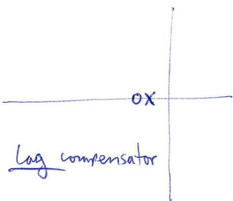
Instead of boosting the phase at  $\omega_c$  to increase PM, we can instead try to decrease gain to improve GM and also shift  $\omega_c$  left (slower) so that PM improves. We do this with a lag compensator.
